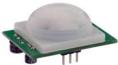
Fig.4. PIR Motion Sensor
